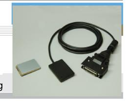
The Dentron image sensor is ideal for intra-oral X-ray imaging in dental diagnosis. The size #2 (1700 × 1200) pixels & size #1 (1500 x 1000) pixels size of 20 × 20 µm. The fiber optic plate (FOP) used as an input window is as thin as 1.5 mm but highly resistant to X-ray irradiation, making the Dent sensor very reliable even over a long-term operation. The scintillator coated on the FOP is optimized to have high X-ray sensitivity and high resolution (20 Lp/mm).
